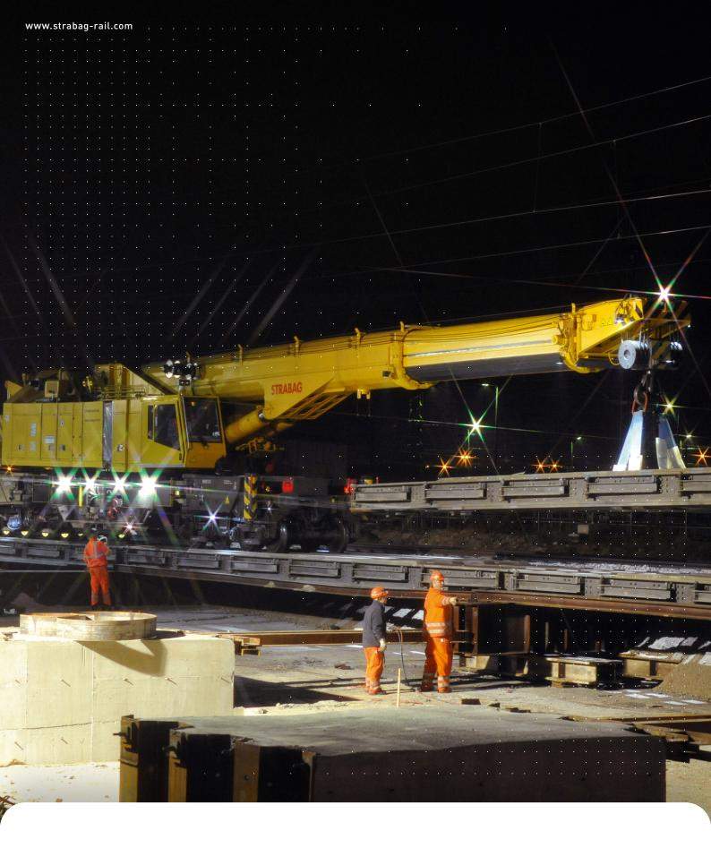
KRC 1200+ TRACK AND TURNOUT CONSTRUCTION CRANE
